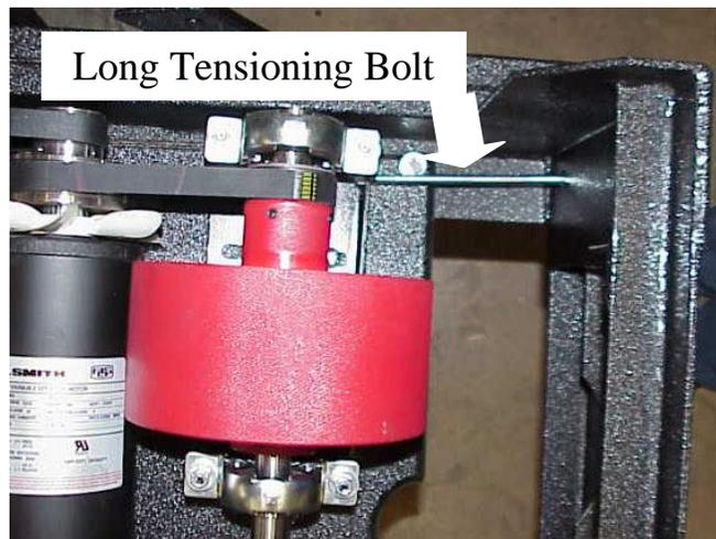
Use a ½” socket wrench to tighten the tensioning bolt just enough to remove the belt slipping. Check the tension on the belt that runs from the motor to the front roller by twisting or wiggling it. You should be able to twist the belt about 90 degrees.
