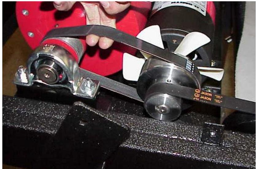
When the flywheel belt has been loosened to the correct tension, tighten the four bolts that hold the flywheel to the floor of the motor compartment.
