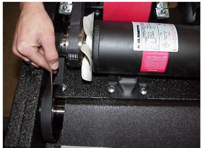
If you wiggle the belt up and down, there should be at least ½” of play. Be careful not to over-tighten the motor belt. **Over-tightening the motor belt will cause the motor shaft to snap and void the warranty.**
